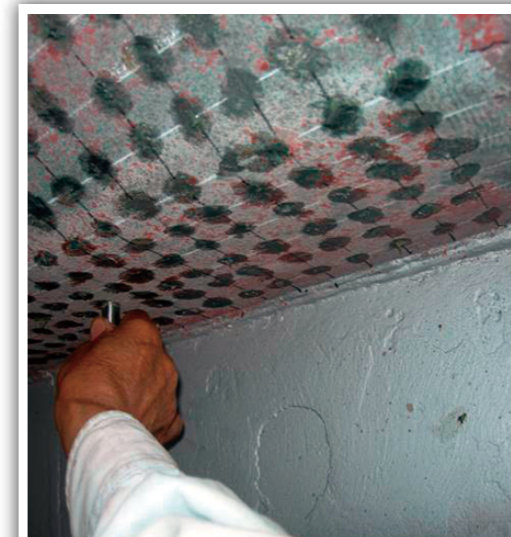
Measurement of bottom shell thickness for aged deterioration
